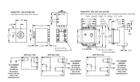
The class 1 model GFM Ground Fault protection systems are designed to minimize damage or loss to equipment caused by destructive arcing ground faults. This GFM systems is designed for all polyphase applications and is ideally suited for motor control, motor control centers, and medium voltage starters. System can be wye or delta, ground or
