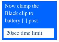
NOTE: 20 seconds is given to establish the contact to the battery [-] post failing which the data obtained earlier will be lost. Then you need to repeat the whole testing procedures again.
