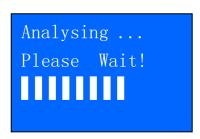
17. Once it has finished analysing, it will prompt you with an instruction stating that you have should unclamp the Black tester clip from the engine or chassis body and transfer to the battery negative [-] terminal within 20 seconds time limit if not the testing procedure has to be repeated again as the gathered data will be lost.
